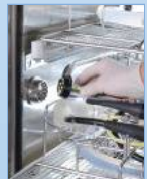
Connecting the CMS adapter.
