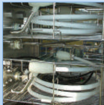
Innova E5 chamber with two endoscope capacity on each of the load carriers.
